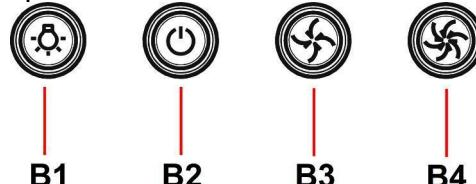
The hood is fitted with a control panel with aspiration speed selection control and a light switch to control cooking area lights.
