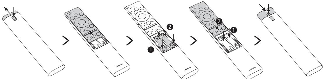
1. Press the at the top rear of the Samsung Smart Remote. The body will pop out slightly from the body cover.
